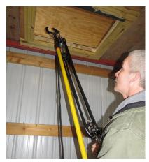
6. Push the Claw opening firmly against the board with the pole. While keeping steady pressure against the board using the pole, firmly grab all the lift ropes and pull the ropes downward. This will securely attach the Claw to the board.
