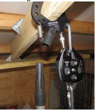
8. Pull ropes again to ensure the Claw is locked on to the board
