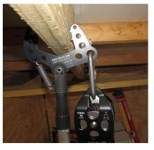
7. With a slight counterclockwise twist, remove the pole and set it aside
